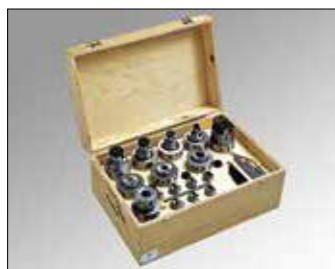
Cod. 9459210 (CM4) – Cod. 9459212 (ISO 40): Box containing taper shanks for end and face-mills, gripper-carrying spindle for 4-20 dia. mm drills, 70 dia. mm boring head with MT4 taper, ISO 40 taper.
