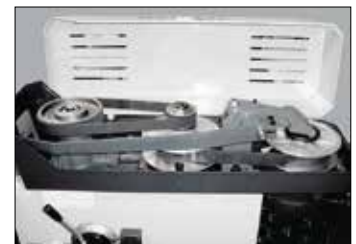
VS: Variable speed-drive unit.
