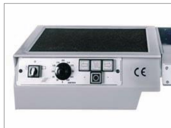
Code 40005: Electronic longitudinal cross table-feed for TC 36÷380 mm/min. Rapid feed 3 m/min
