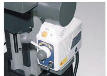
Code 40026 Power: Power Mechanical longitudinal cross-table feed
