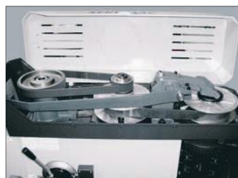
VS: Variable speed-drive unit
