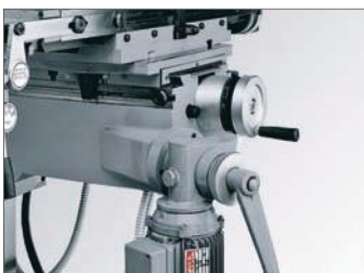
Code 40006: Rapid vertical table feed
