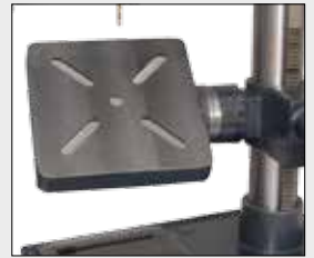
PG: 230 x 230 mm Rectangular table with rack
